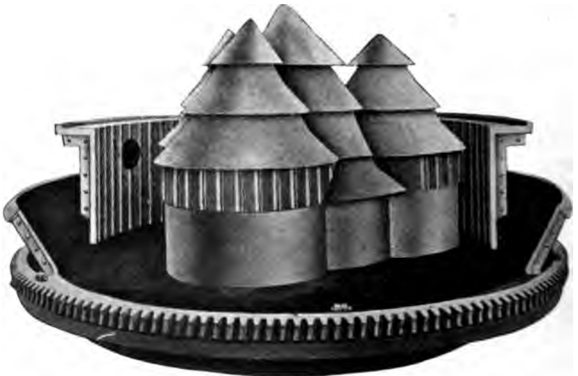
FIG. 248.—Rehmann revolving eccentric grate.
